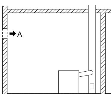
$$A = 150 \text{ см}^2 + 2 \frac{\text{см}^2}{\text{кВт}} \times (\Sigma Q_n - 35 \text{ кВт})$$
